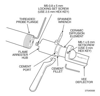
Figure 4-5. Ceramic Diffusion Element Replacement
